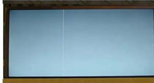
Vertical Line Source TAB IC Defect
